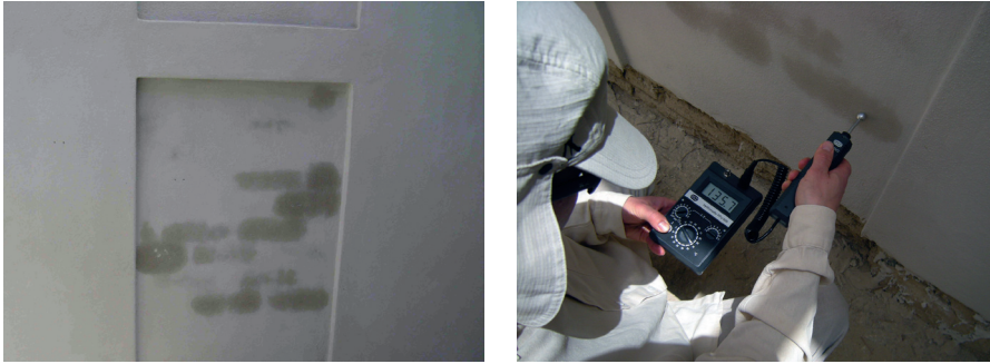
Fig. 2.8 : Dark patches indicate hygroscopically induced moisture resulting from the use of earth blocks with high salt content. Right: measuring the moisture content (Jahili Fort, Al-Ain, UAE)
