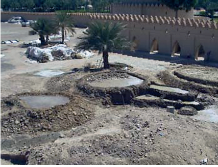
Figs. 2.7 a and b : Salt effluorescence visible on reproc- essed earth from soaked demolition material (Jahili Fort, Al-Ain, UAE)
